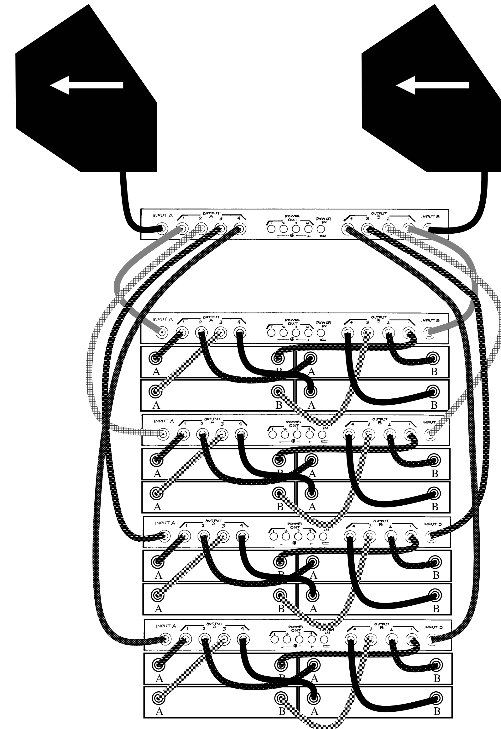
SIXTEEN RECEIVERS WITH FIVE SPLITTERS AND TWO ANTENNAS
